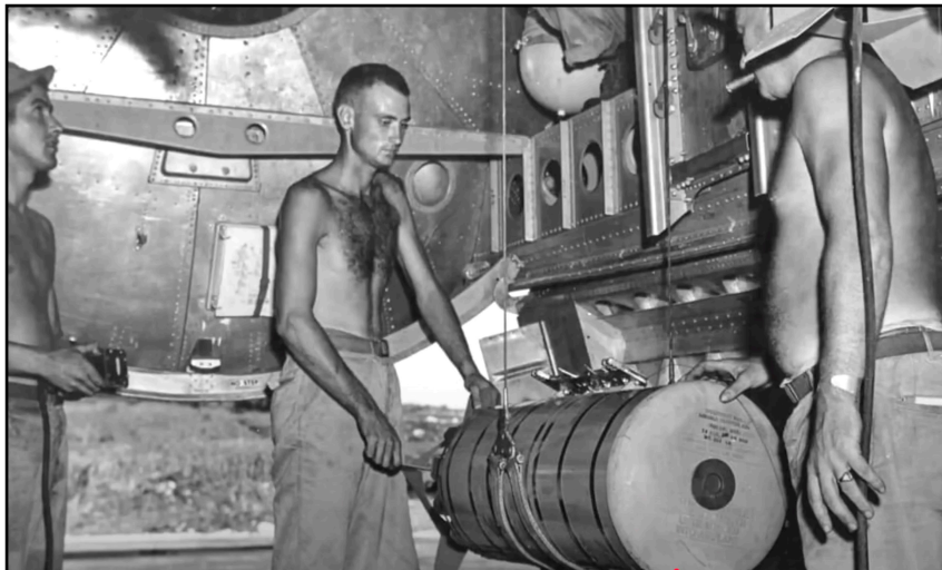
A B29 munitions crew winches an E-46 up and into the bomb bay. Each Superfortress carried forty such bombs which gave them the capacity to deliver 1520 individual bomblets over their target.
